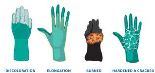
Degradation is also a key factor which needs to be taken into account. Chemicals can degrade materials in many ways, all of which can potentially affect the protective properties of the PPE. Examples of degradation include discoloration, elongation, burning, hardening, and cracking. If any of these are present it is recommended that the PPE is replaced.
